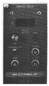
0.2 TO 48 MSEC DELAYS, CONTINUOUSLY VARIABLE
